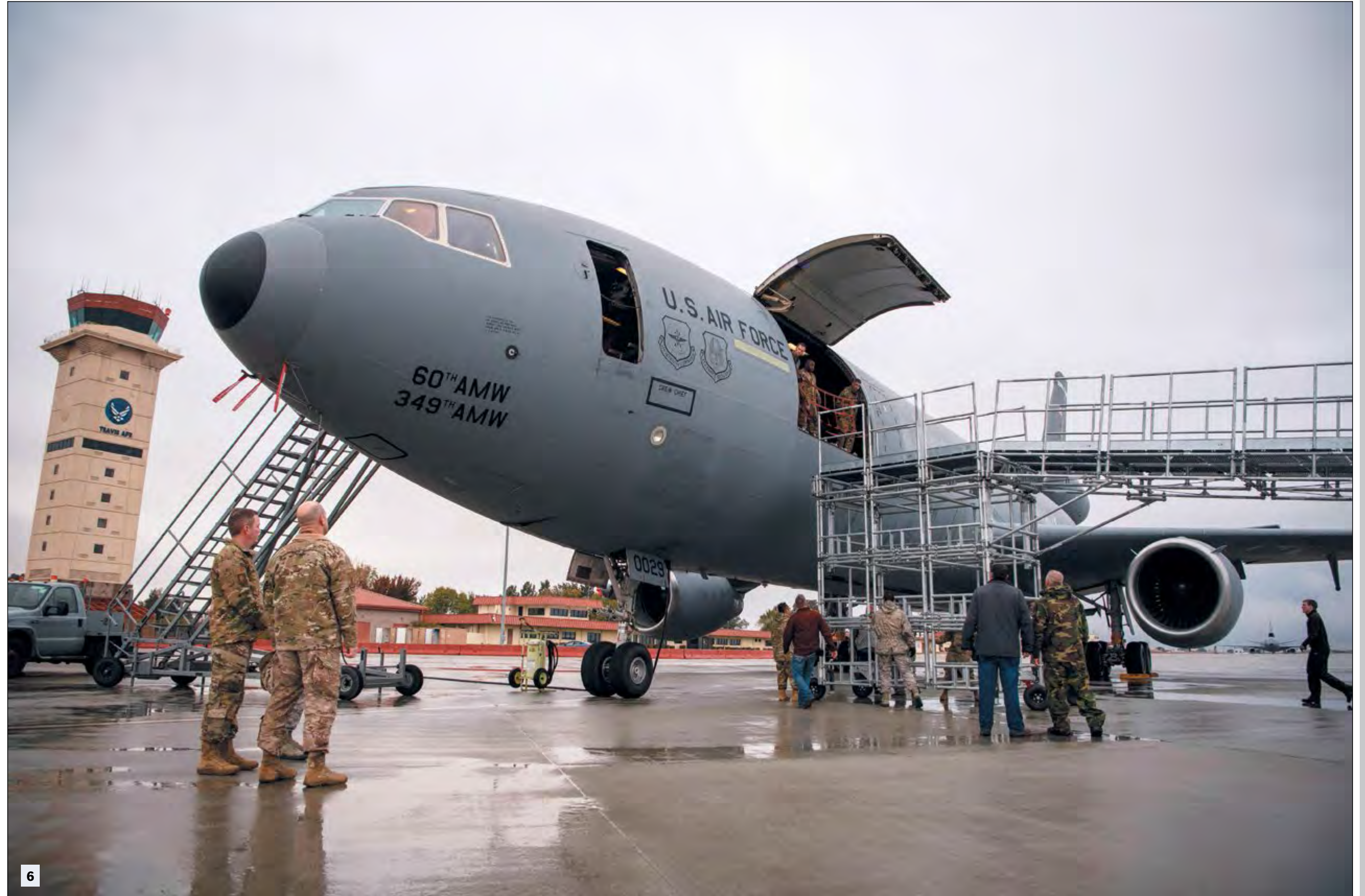
U.S. Air Force photos/Nicholas Pilch 1) U.S. Airmen from the 60th Medical Readiness Flight install a prototype patient loading system for the KC-10 Extender Dec. 4 at Travis Air Force Base, California. Airmen built and tested the system to meet Air Force standards and upgrade from the current system. 2) Airmen transport a simulated patient on a prototype patient loading system Dec. 4 at Travis. 3) Airmen build a prototype patient loading system Dec. 4 at Travis. 4) Staff Sgt. Shae Nagamine, 60th Medical Readiness Flight medical technician, takes a break from building a prototype patient loading system Dec. 4 at Travis. 5) Airmen from the 60th Medical Readiness Flight build a prototype patient loader for the KC-10 Dec. 4 at Travis. 6) Col. Jeff Nelson, left, 60th Air Mobility Wing commander, and Col. David Hammerschmidt, 60th Maintenance Group commander, watch Airmen install the prototype Dec. 4 at Travis.
