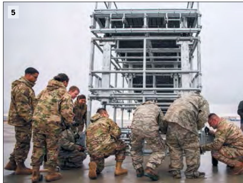
U.S. Air Force photos/Nicholas Pilch 1) U.S. Airmen from the 60th Medical Readiness Flight install a prototype patient loading system for the KC-10 Extender Dec. 4 at Travis Air Force Base, California. Airmen built and tested the system to meet Air Force standards and upgrade from the current system. 2) Airmen transport a simulated patient on a prototype patient loading system Dec. 4 at Travis. 3) Airmen build a prototype patient loading system Dec. 4 at Travis. 4) Staff Sgt. Shae Nagamine, 60th Medical Readiness Flight medical technician, takes a break from building a prototype patient loading system Dec. 4 at Travis. 5) Airmen from the 60th Medical Readiness Flight build a prototype patient loader for the KC-10 Dec. 4 at Travis. 6) Col. Jeff Nelson, left, 60th Air Mobility Wing commander, and Col. David Hammerschmidt, 60th Maintenance Group commander, watch Airmen install the prototype Dec. 4 at Travis.
